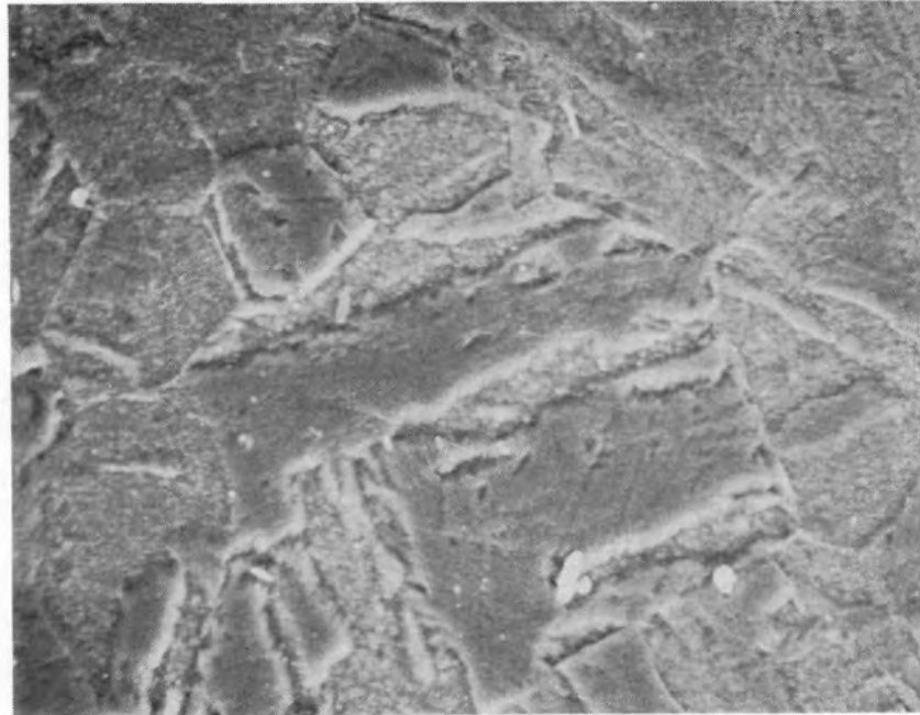
Figure 19. SEM micrograph of Sample 7a (304 SS) microstructure.
